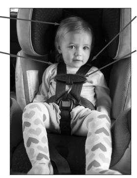
Harness should be at or below shoulder level and threaded correctly.
