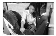
There are two different seat belt paths in a convertible car seat. One is for rear-facing and one is for forward-facing. The correct belt path must be used based on the direction the car seat faces.
